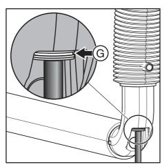
7. Snap the retaining ring into the groove (G).
