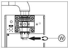
**3.** After insertion, secure the support arm with a retaining ring (**W**) to prevent it from getting lifted out.
