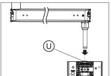
**4.** Thread the threading aid through the bearing. Position the support arm in the bearing (**U**).
