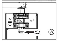
**5.** After insertion, secure the support arm with a retaining ring (**W**) to prevent it from getting lifted out.
