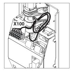
Roll up the extra lengths of cable L1 and of the grounding strap to the right of the bearing block and secure the cable roll with a cable tie on the cable clamp.
