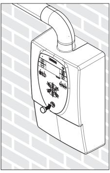
**3. Only with manual release S3 (coiled cable):** Cover the release symbol on the control membrane with the adhesive dot provided.
