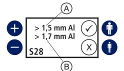
By pressing the +/- button, the filter setting can be amended between 1.5 mm AL and 2.5 mm AL in 0.1 mm steps.
