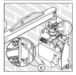
**10.** Check the support arm with the spirit level. If necessary, loosen the bearing mount (4 nuts) and place the shim (**X**) underneath.
