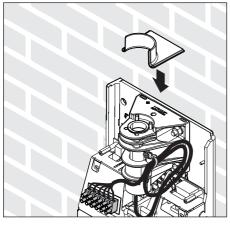
**3.** Set the cover of the arm connection onto the wall module as shown, between the support arm and the wall.
