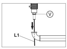
**5.** Route the arm cable (**L1**) downwards through the arm and insert the scissor arm. Make sure that the washer (**V**) does not fall off during this step.
