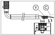
**10.** Thread the ferrite core (**Y**) **only** onto the arm cable (**L1**) and slide the ferrite core into the support arm.
