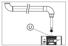
2. Insert the support arm into the bearing (U).
