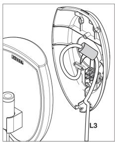
1. Only with manual release S3 (coiled cable): Place the ferrite core of the coiled cable inside the housing.
