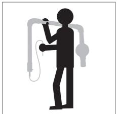
**4.** For transport and for the next installation step, support the scissor arm on your shoulder.
