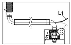
**9.** Disconnect the arm cable (**L1**) and the grounding strap (**C**) in the accessible area.
