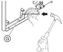
**8.** "Elongated hole" installation version only: Carefully punch out opening (G) in the wall adapter with a punch.
