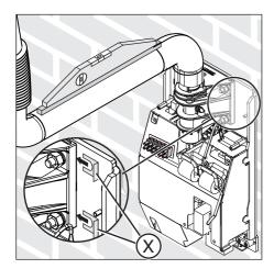
**13.** Check the support arm with the spirit level. If necessary, loosen the bearing mount (4 nuts) and place the shim (**X**) underneath.
