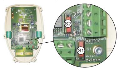
The safety circuit can be bypassed via hardware on DX4 (slide switch S2) (See section "Setting switch S1 and S2 on DX4 [  $\rightarrow$  76]".
