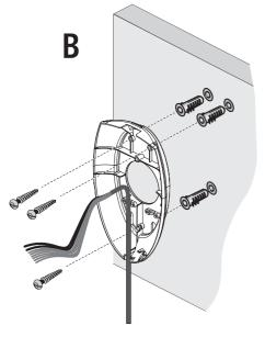
**3.** Fasten the chassis firmly to the wall with three screws.
