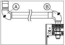
2. Attach the housing shells **A** and **B** to the support arm.
