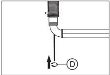
**6.** Push the retaining ring (**D**) through the arm cable
