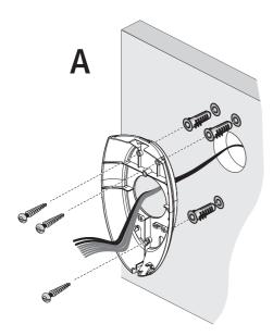
2. Drill the holes (6 mm (1/4") masonry drill bit) and insert the wall plugs.
