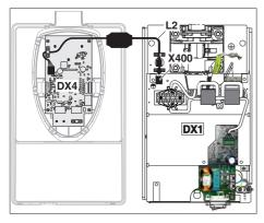
2. Secure power cable L2 with the strain relief (K).
