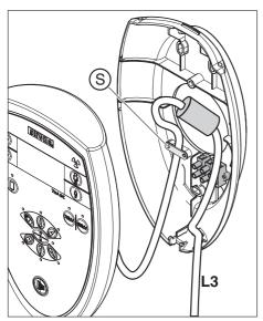
1. Only with manual release S3 (coiled cable): Place the ferrite core of the coiled cable inside the housing centered on the opening in the wall. To do this, fasten the coiled cable with the strain relief clamp (S).
